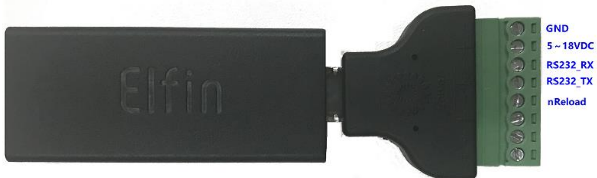
Figure 8. EW10 +8PIN Connector
