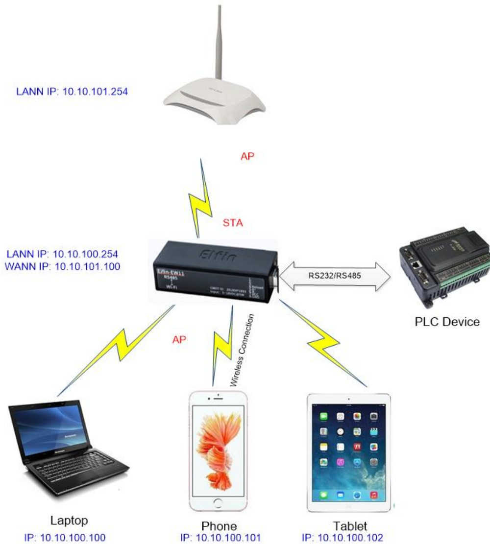
Figure 25. AP+STA Wireless Network
