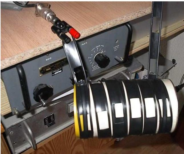
Fig.2 Example of an ,airwound' Balun
