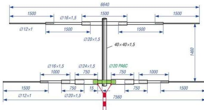
Fig. 5 Structure of the antenna
